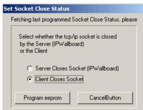
Figure 5-5 Set Socket Close Status window
