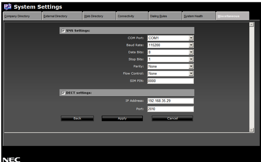
Figure 8-41 Miscellaneous window - Configure Messaging Service
